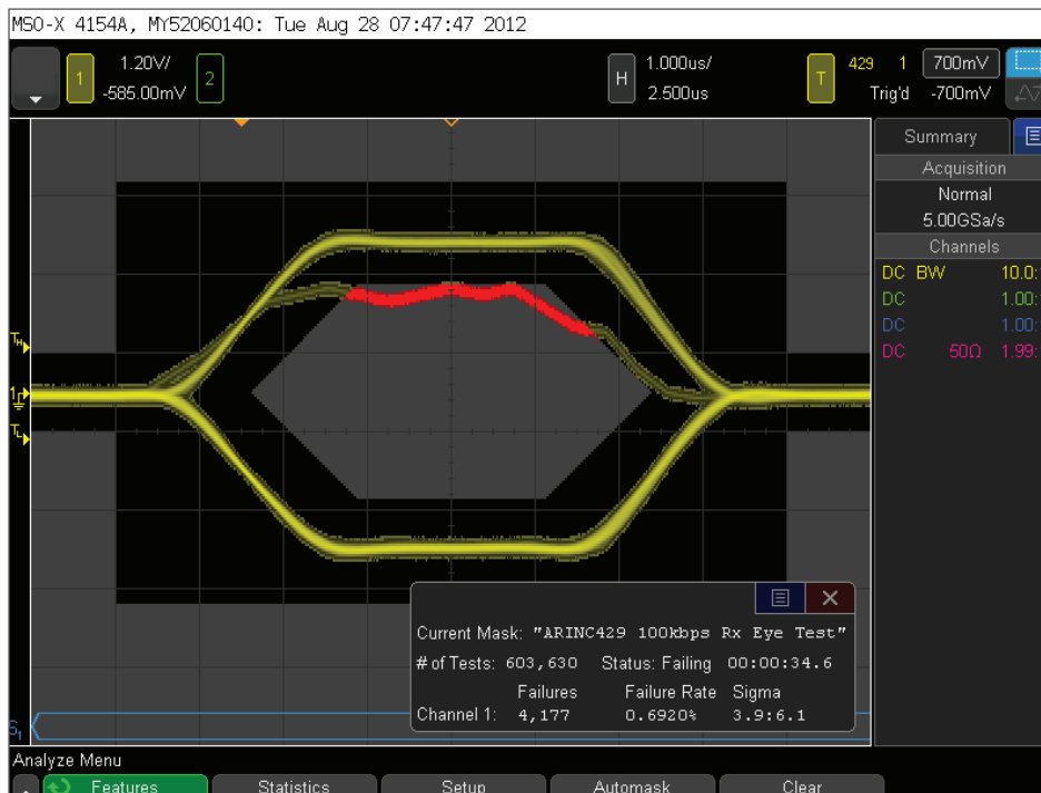
Figure 4: Mask testing lets you specify areas around your signal that should be off limits
